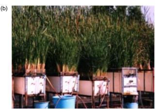
Fig. 5 Domestic wastewater treatment using a wetland system. (a) Co-researchers at the wetland site, (b) Pilot-scale wetland system.
