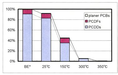
Fig. 2 Extraction of Dioxins in Soil by Hot Water.
