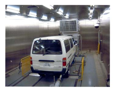
Fig. 1 Chassis dynamometer for automotive exhaust measurements.
