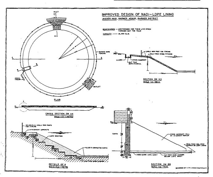
Fig. 10 Improved design of nadi with LDPE lining developed by CAZRI, Jodhpur.
