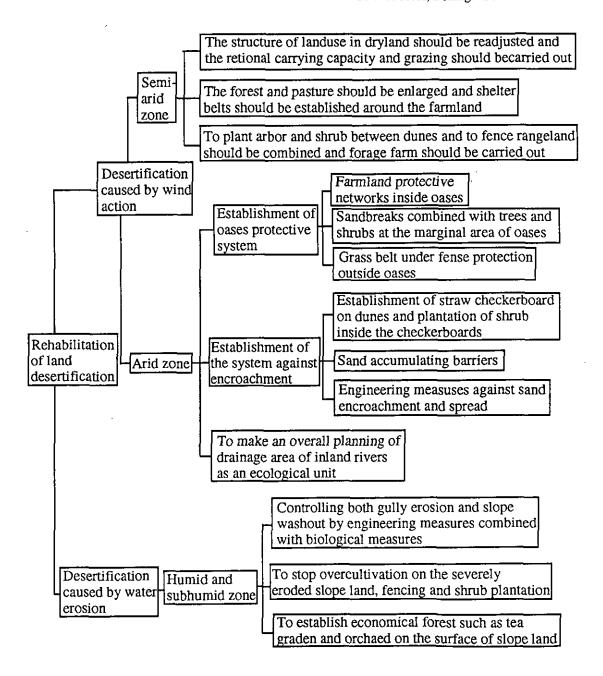
Fig. 3 The Measures for Combating Desertification in China.
