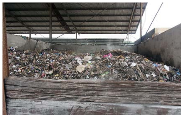
Fig. 37 Aerobic fermentation at a composting plant in Hanoi City, Vietnam
