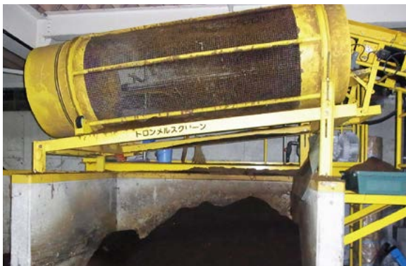
Fig. 28 Trommel to remove contaminants after the fermentation process in Ikeda Town, Japan
